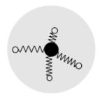
Classical model of an atom. Electrons are bound to the nucleus by springs which determine the natural frequencies.
