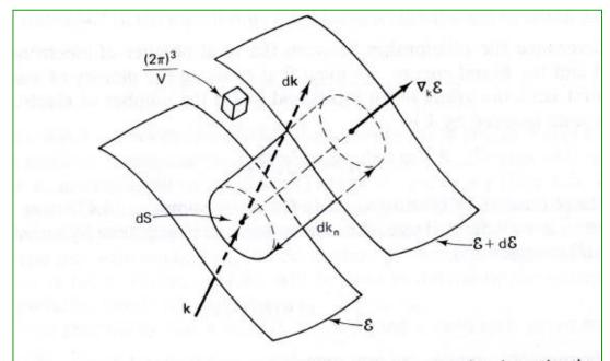
Figure 4.3 Diagram of the vectors and differential volume used to determine the density of states in the first Brillouin zone.
