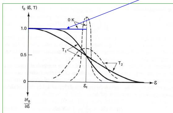
Figure 4.2 The equilibrium Fermi-Dirac distribution function and its energy derivative (dashed lines) for  $0 < T_1 < T_2$ . The derivative at 0 K is a delta function.
