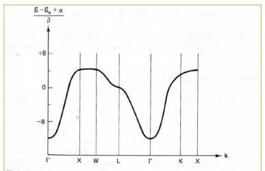
Figure 2.12 Tight-binding energy band, corresponding to one atomic state, for a face-centered cubic lattice with a basis of one atom.
