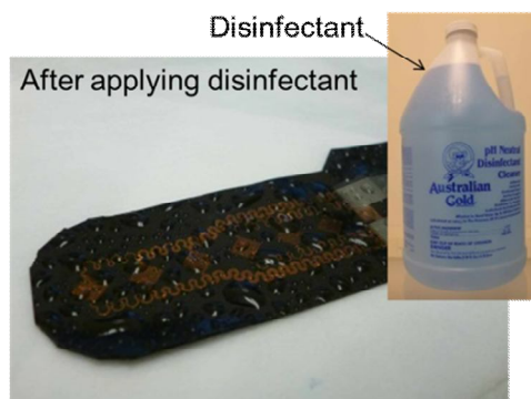
Figure S19. Photo of an EES after spraying with a disinfectant solution (pH Neutral Disinfectant Cleaner, Australian Gold, Indianapolis, IN, USA) for device cleaning.
